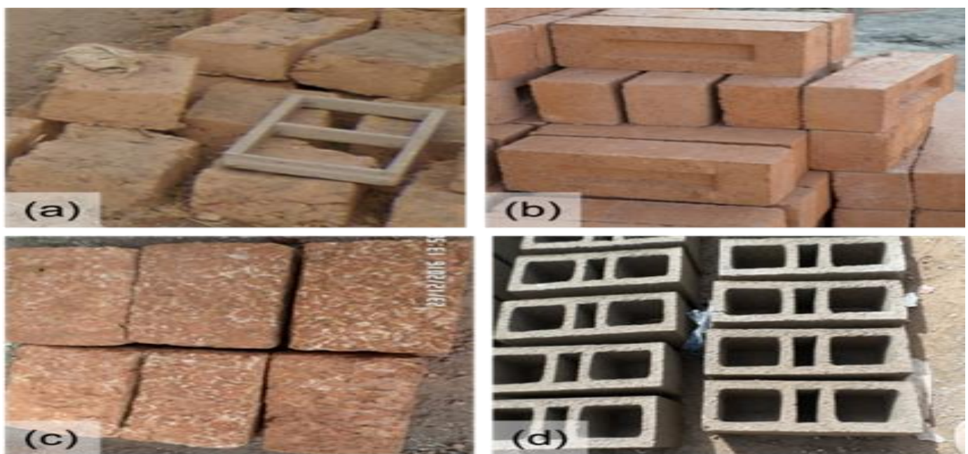
Figure 1. Different types of masonry bricks used in construction in Ouagadougou : a) adobe bricks, b) compressed earth blocks, c) cut laterite blocks (BLT), and d) cement blocks (ZOUNGRANA, field survey 2017 and 2018)
